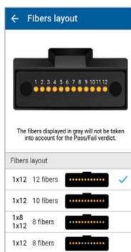
Pass/fail thresholds according to fibers layout selection
