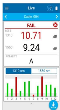
Power meter main screen
