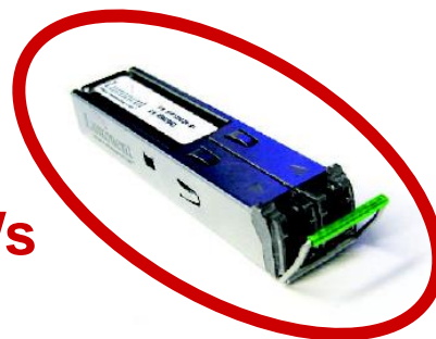
SFP+ transceiver (Small Formfactor Pluggable) LC duplex
