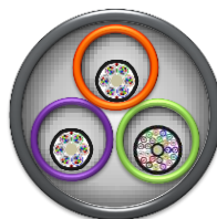
Total Capacity: 3 x 96FC Microduct : 12/10 (diameter / bore)
