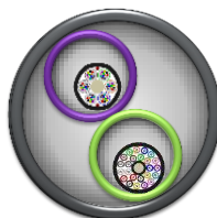
Total Capacity: 2 x 96FC Microduct : 14/12 (diameter / bore)
