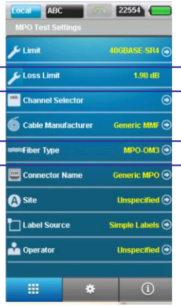
Based on the fiber type, OM3/OM4 and the application selected, the loss limit is applied.
