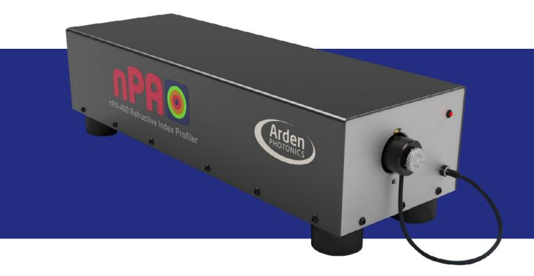
The nPA-400 Refractive Index Profiler uses a modified refracted near-field technique to analyse a fiber end-face to determine the full 2D refractive index distribution. The nPA-400 is the quick and easy way to get the Refractive Index data you need to verify your specialty fiber design and manufacturing processes.
