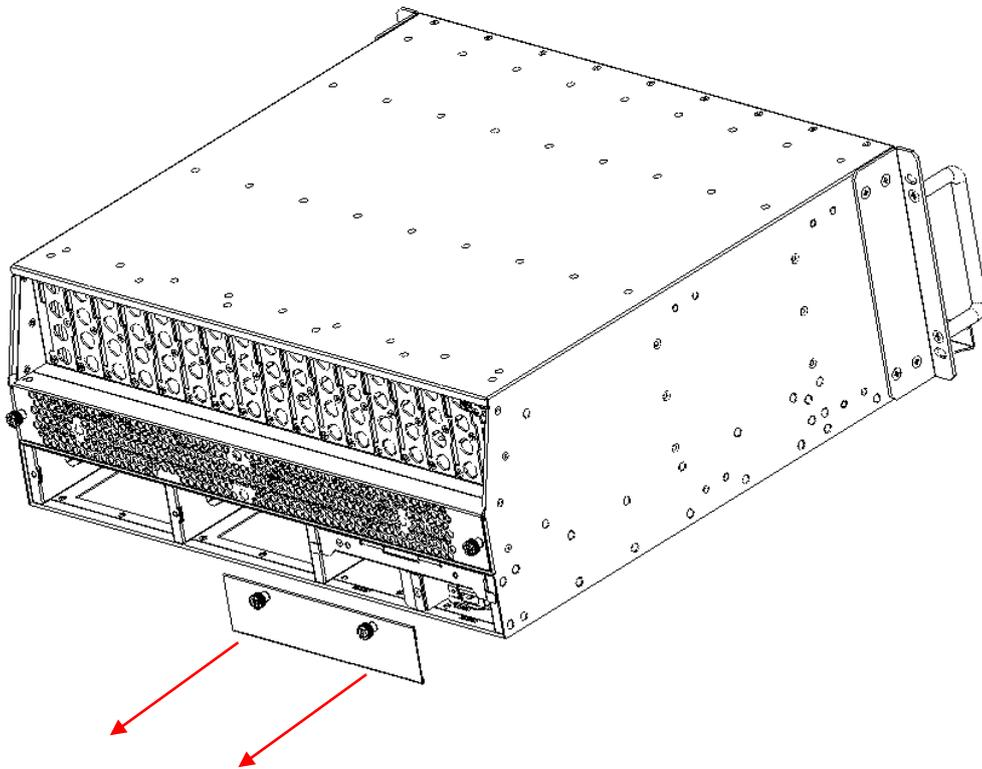
3. Then lift up the handle and slide the fiber guide out of the front of the chassis.
