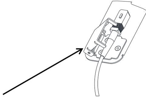
When using the sliding guide, put the fiber connector in the clip and slide it in from the rear to the front, through the chassis. Ensure that the optical fiber tail does not become trapped or pulled tightly.
