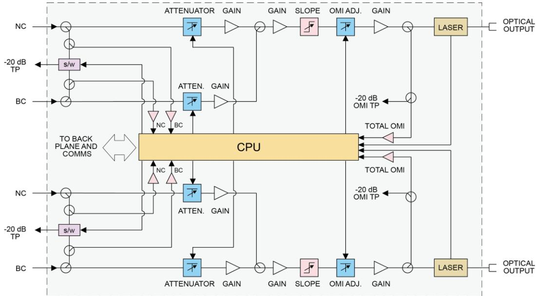
Figure 3-1 Block diagram FT5S
