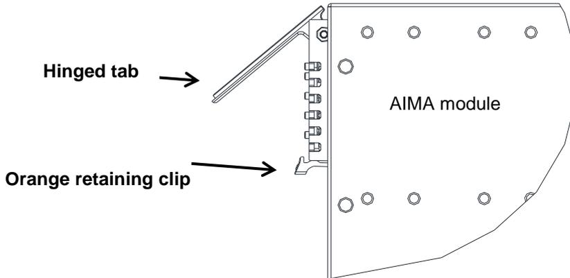
2. Hold the AIMA module casing upright, align it with the AIMA3000 slide rails for the correct slot, and insert the module until it reaches the multi-pin connector.
