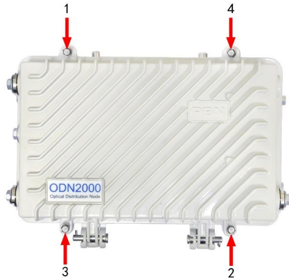
Figure 5-8 Screw Tightening Order
