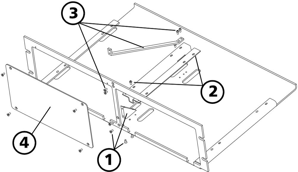
2. Fix the rackmount bracket to the frame using two round Phillips screws.
