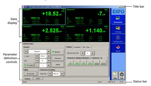
**Note:** When using a multichannel power meter with different optical heads, the settings (such as the wavelength list) used by the application are those detected on the highest channel number. For example, if you use a Low-PDL head on channel 2 and a high-power head on channel 3, the high-power head settings will take precedence. If you move the head from channel 3 to channel 1, the Low-PDL head will be used for settings instead.
