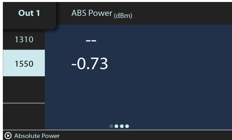
Figure 10: BR1 Absolute Power page – live reading
