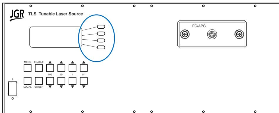
Once all is set properly, then pressing the BEGIN SWEEP key will start the sweep sequence which will automatically stop once the STOP wavelength is reached.
