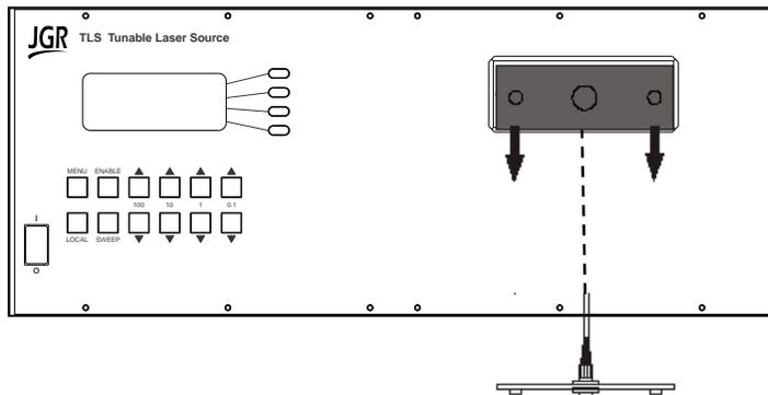
Figure 5: Removing Connector Panel
