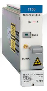
Cost effective, external cavity tunable laser modules utilizing a patented T100 cavity. Minimum of 100 nm tuning range with narrow linewidth, high output power and ultra-low optical noise (significantly increases measurement dynamic range). Its kinematic chain has been designed for step-by-step wavelength tuning.
