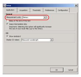
**4.** If you would like the unit to warn you when a test is complete, select the corresponding option.
