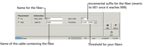
**Note:** The fiber name, cable ID and automated additions to the file name such as the date can be set in the **Preferences** tab of the **Setup** window. See Setting Test Preferences on page 38 for details.
