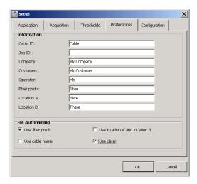
**4.** If you want the application to automatically include the fiber prefix, cable name, A and B location or date in the file name scheme, select the corresponding option.
