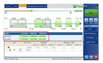
When a multiple-wavelength acquisition is in progress, only the wavelength currently being acquired and the ones already completed are displayed. Link loss, link ORL, and propagation delay (multimode only) are displayed for each wavelength. For the link loss and the link ORL, the values are tested and displayed according to current pass/fail settings.
