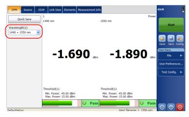
The power levels are displayed for the selected wavelength in the **OPM** tab.
