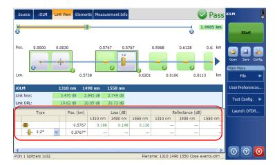
Elements diagnostics are associated with specific link elements issues. Each failed link element will have associated diagnostics to assist in troubleshooting. Some elements, such as macrobends, will have associated diagnostics even with a pass status.
