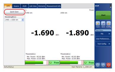
The power level is saved into a file, the file name is displayed in the status bar.
