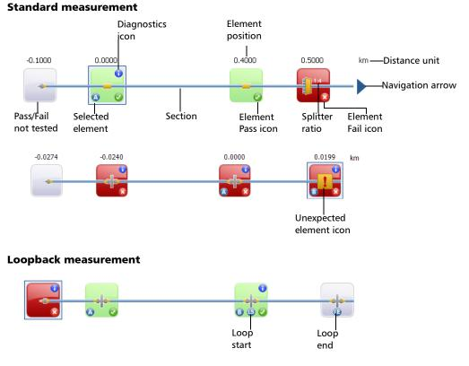
Element position: The distance of the element from the beginning of the link under test.
