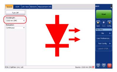
3. Select the desired modulation from the Modulation list.
