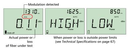
When the unit detects a modulated signal, it beeps and displays the modulation value and *average* measured power or loss (see left illustration above). You may notice a slightly unstable last digit.
