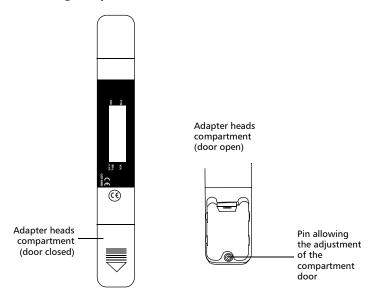
The LFD-201, LFD-202 and LFD-202P Live Fiber Detector are supplied with three adapter heads:
