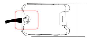
With a flat-head screwdriver, press down on the small silver ball until the head of the screwdriver fits into the small grooves on each side of the screw.
