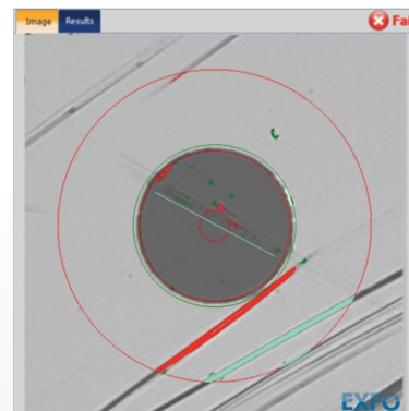
Damaged=must replace the connector
