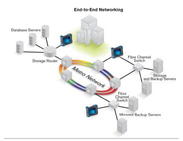
Thanks to end-to-end network testing capabilities, EXFO's NetBlazer enables fast deployment and configuration of Fibre Channel networks. Communication between the transport network, interconnection devices and end nodes can be validated with features such as BER testing, latency measurement, buffer-to-buffer credit estimation and port login capabilities.
