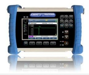
Ether10. Dualoop is a battery operated 10 Gbit/s loop-back device with two optical/electrical ports that can loop back Ethernet/IP L1-L4 packets sent to execute acceptance and assurance tests including RFC2544 or eSAM.
