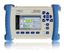
Net.Storm is hardware based impairments generator, equipped with double GbE ports, battery operated, fast and full-featured, can emulate the dynamics of real Ethernet / IP networks in terms of packet impairments.
