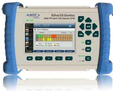
ALBEDO Ether10.Genius is a multitechnology Ethernet tester that includes a Rubidium clock. It is ideal to install / measure advanced telecom services (such as LTE / TDD) at 10GbE, GbE, SyncE, PTP, Jitter/Wander, T1/E1, 1 pps, C37.94, Datacom, OWD.
