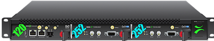
Figure - The 1RU Enhanced Chassis populated with one VB120 module controlling two VB252 DVB-T/T2 input modules giving a total of 4 independent RF inputs.
