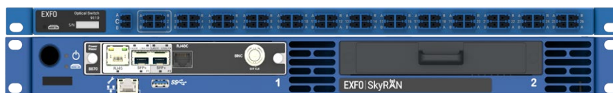
Small C-RAN configuration, duplex, uplink/downlink, 26 ports, 1.5U
