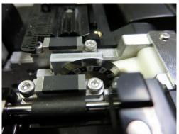
pinch roller with cotton swab soaked in alcohol after each use. After repeated use, abrasion may form on the rubber of the pinch roller. However, the pinch roller keeps the function of collecting optical fiber, as long as the depth of a groove is smaller than the diameter of the fiber. When the function cannot work, even if after cleaning the pinch roller with alcohol, contact local service to replace the pinch roller with a new one at customer's expense. (%1).
