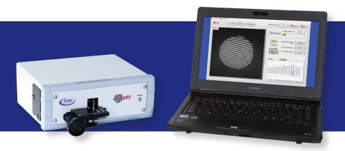
The VFI is an interferometric inspection system specifically designed for checking the surface quality and flatness of your cleaved or polished fibers. The VFI interferometer has proved itself in Research, Production and QA over and over and the feedback we get from users indicates that they value these features:
