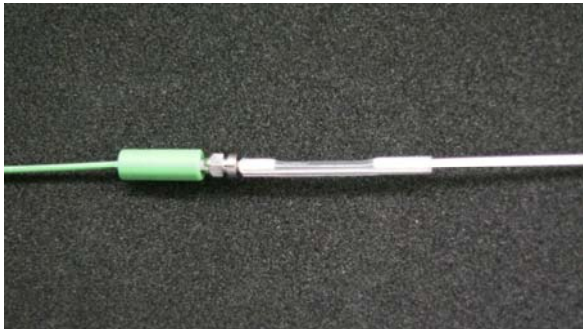
Step 4 Pick up the fiber from the heating stage.
