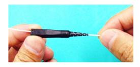
(3) Slide Splice Protection Sleeve onto buffer cord.
