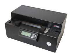
The proven Burst Technology<sup>™</sup> method instantly vaporizes the fiber coating. The result is a clean, stripped fiber, at substantially higher strength than any mechanical stripping method. The fiber is free of debris at 400x magnification. The AutoStripII is also equipped with a built-in, high force, fiber tensile tester, which can pull the fiber up to 235 kpsi (20 N).
