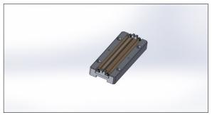
Silicon Mould, Mould Holder & Fiber Guide
